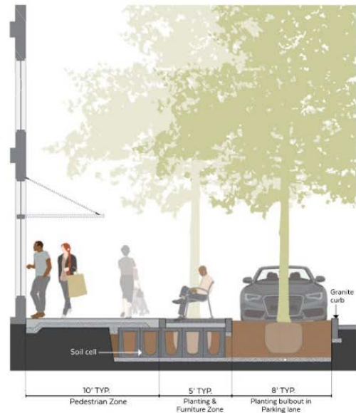
WIDE SIDEWALK (>10 feet wide) SECTION
