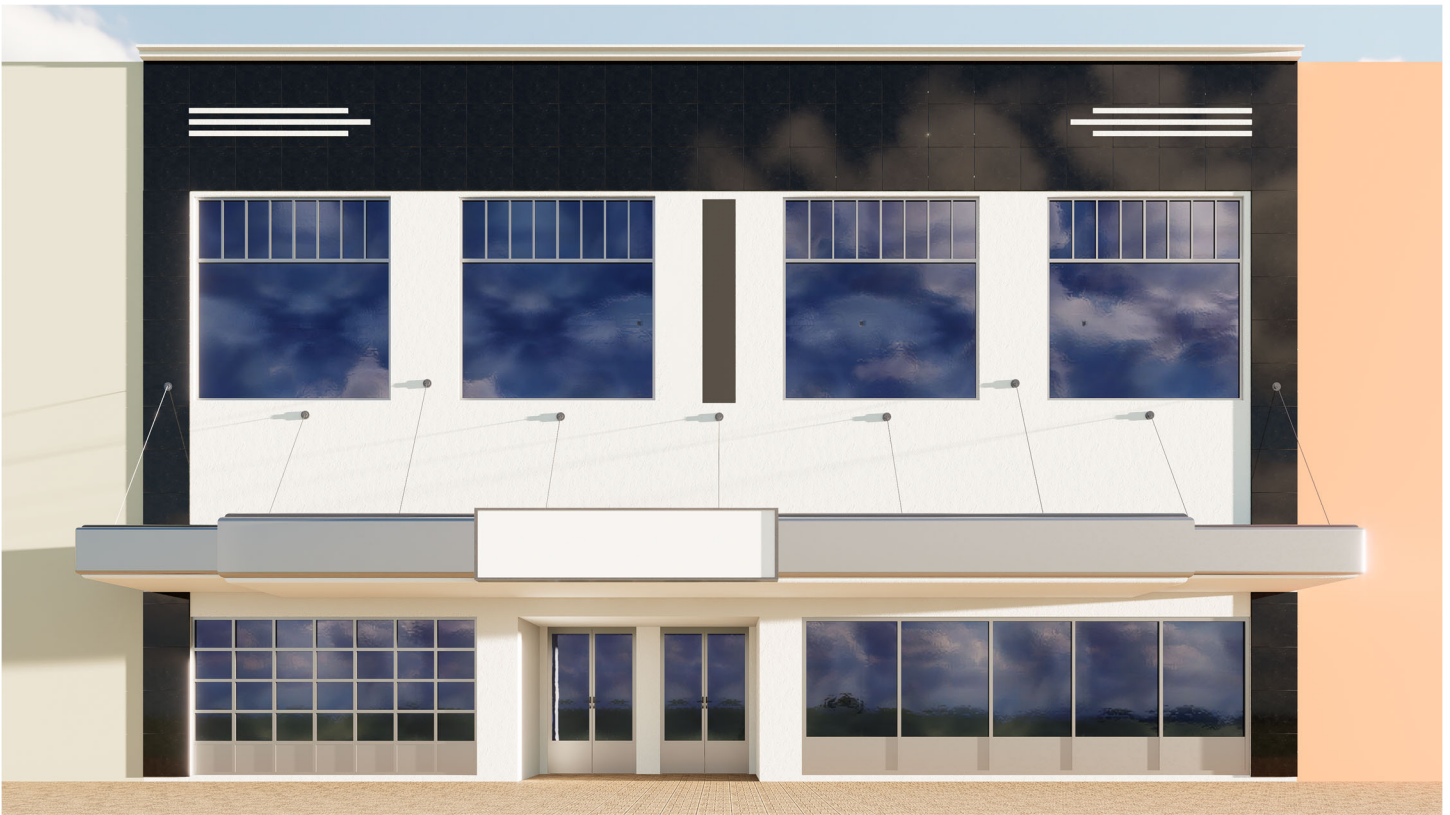
Rendering shows the unified central color of white, Black vitrolite on the ends to the ground to anchor the 2 levels together. The rendering was made prior to the final alteration to include bifold panel doors at both tenant storefronts.
